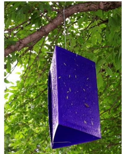
Sticky insect trap used to sample for EAB.
